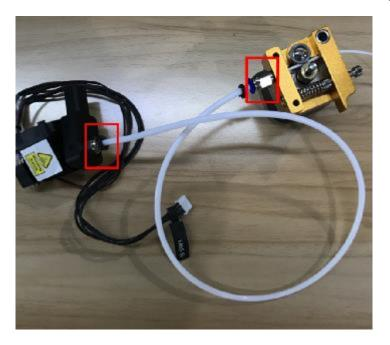
Figure 5.78 Connect extruder and hot end
