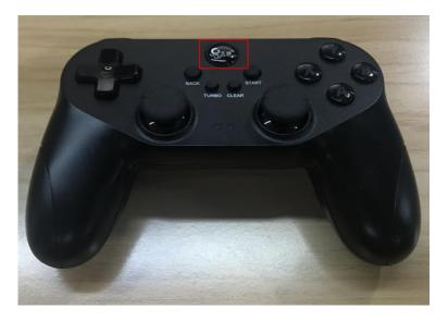
Figure 5.140 Power button of the stick controller
