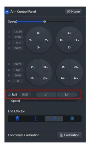
Figure 5.39 Enable sliding rail
