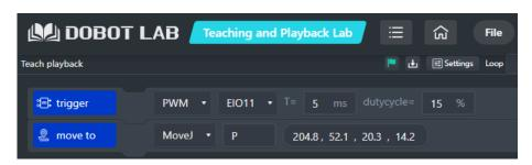
Figure 5.151 Move the trigger command
