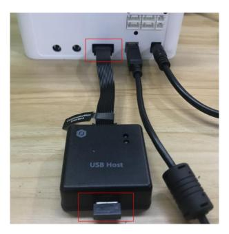
Figure 5.138 Connect with USB Host module
