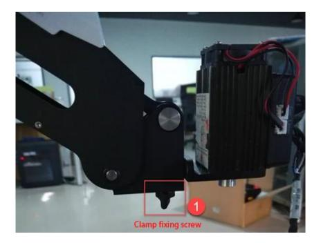
Figure 5.52 Fasten the laser with clamp fixing screw
