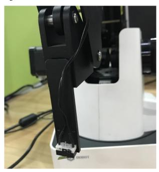
Figure 5.129 Fix auto-levelling tool
