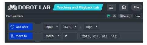
Figure 5.149 Move the trigger command
