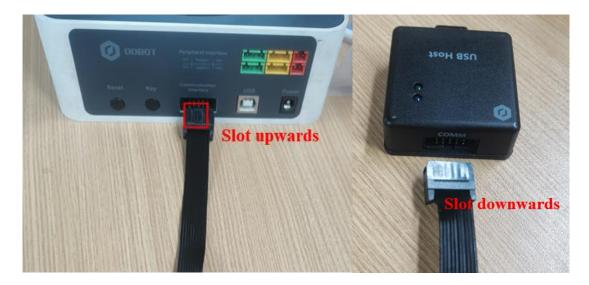
Figure 5.139 Connect Magician to USB host
