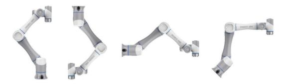
Figure 7.1 CR robot installation posture
